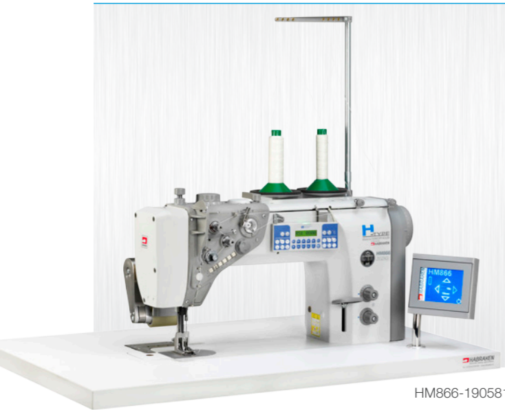
Touch panel zigzag selector
