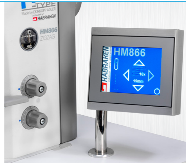
Touch panel zigzag selector
