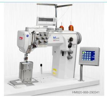
Special machine for sewing decorative stitches based on a Dürkopp Adler M-Type customized by Habraken.
