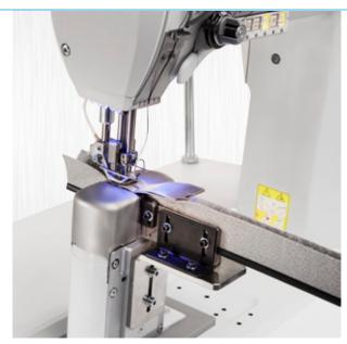
With this retro fit kit it is possible to rebuild a standard Dürkopp Adler 868 or even the older 768 post bed machine for attaching a double flag PWP extruded listing underneath upholstery pieces.
